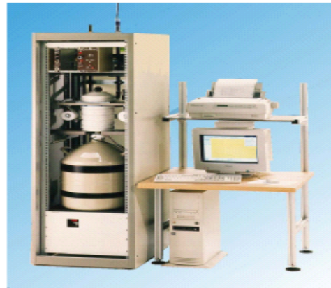
Figure C-2: The Nuclide specific detection of gamma emitting radionuclides Unit (20) .
