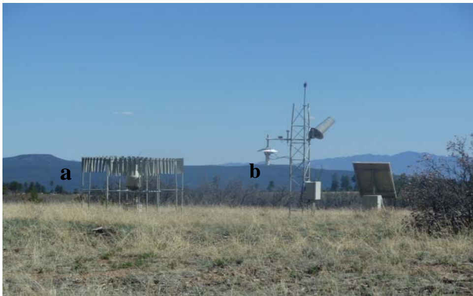
Figure B-1: Example of NEWNET station (south of LANL near Bandelier National Monument) where we can find (a) rain sampler and (b) air sampler.
