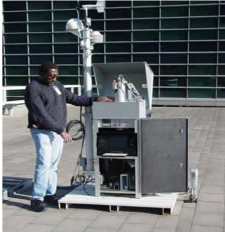
Figure 3: Example of radiation monitoring station developed by US EPA RadNet. The system includes meteorological data collection (24) .
